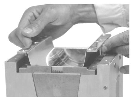
Figure 23. Reflector Removal or Replacement (I300M)
